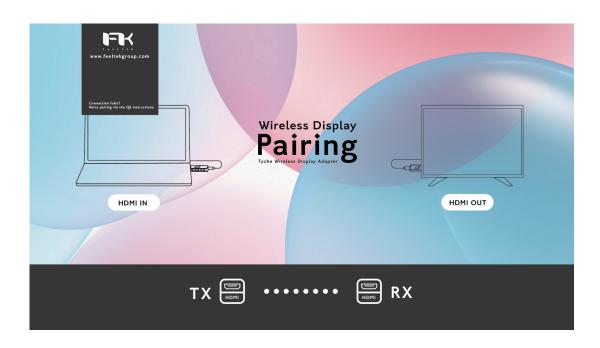
Wait for the device and monitor to detect, while detected the external device will show the pairing screen. TX and RX will automatically pair and once they are successfully paired, the external device will go into the display mode of your connected device
